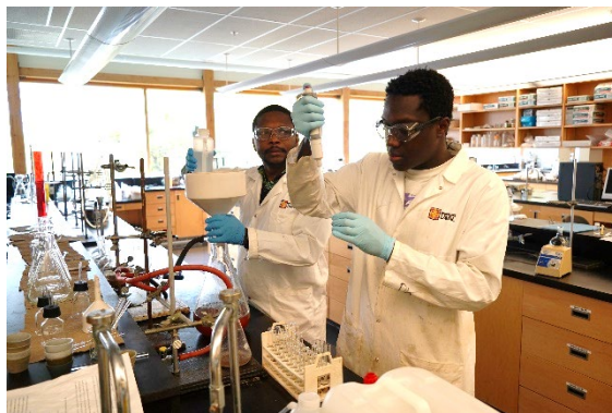
Figure 4: Filtration of organosolv pulp and lignin Klason
