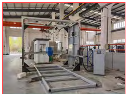
3D Concrete Printer
