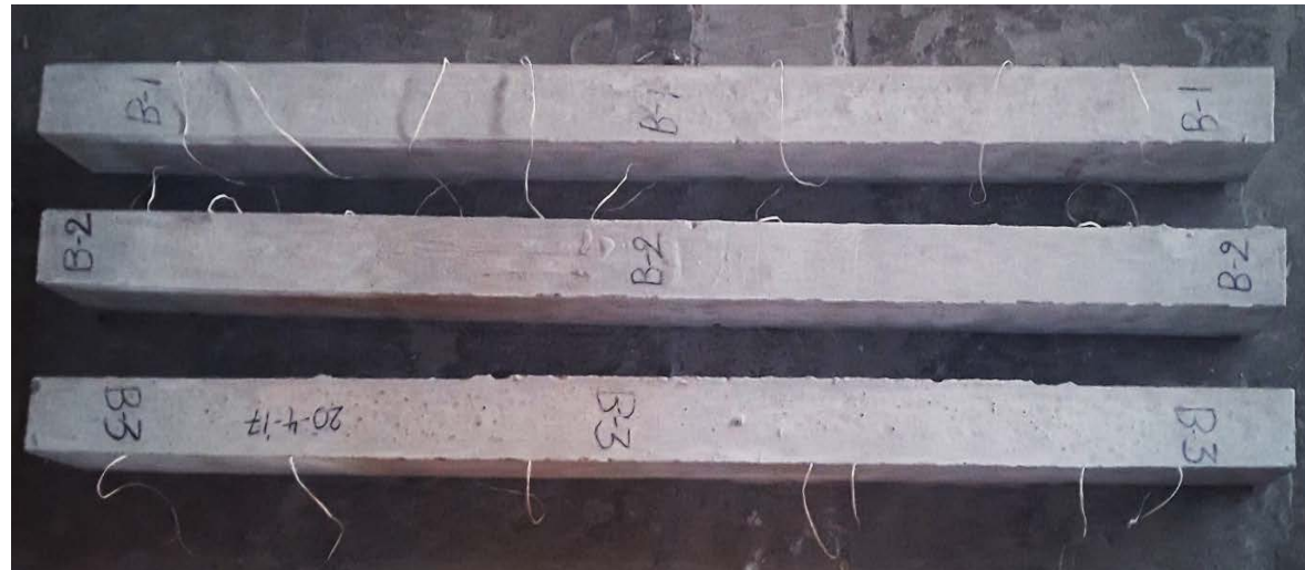
Strain gauges installed on tensile reinforcement
