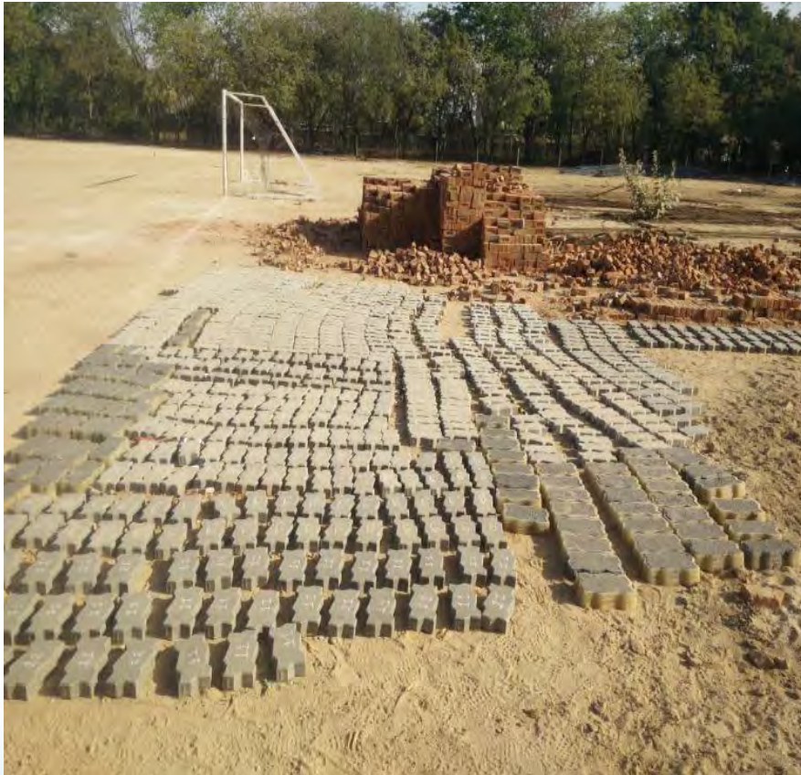
Alkali Activated Concrete Paver Blocks casted in Casting yard at Nirma University
